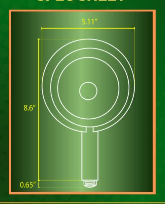
**BUILT WITH SOLID ALUMINUM AND A BRONZE** FINISH, FULLY SEALED FOR ALL-WEATHER **DURABILITY. FEATURES AN INTEGRATED 6W** LED WITH A 3CCT SWITCH (3000K, 4000K & **5000K)**, DELIVERING 500 LUMENS AND A 65° BEAM ANGLE FOR PRECISE, CUSTOMIZABLE LIGHTING. INCLUDES A HEAVY-DUTY GROUND STAKE FOR QUICK AND SECURE INSTALLATION. **IP65** WATERPROOF RATING ENSURES RELIABLE PERFORMANCE IN ANY ENVIRONMENT. IDEAL FOR GARDENS, TREES, AND ARCHITECTURAL HIGHLIGHTS.
